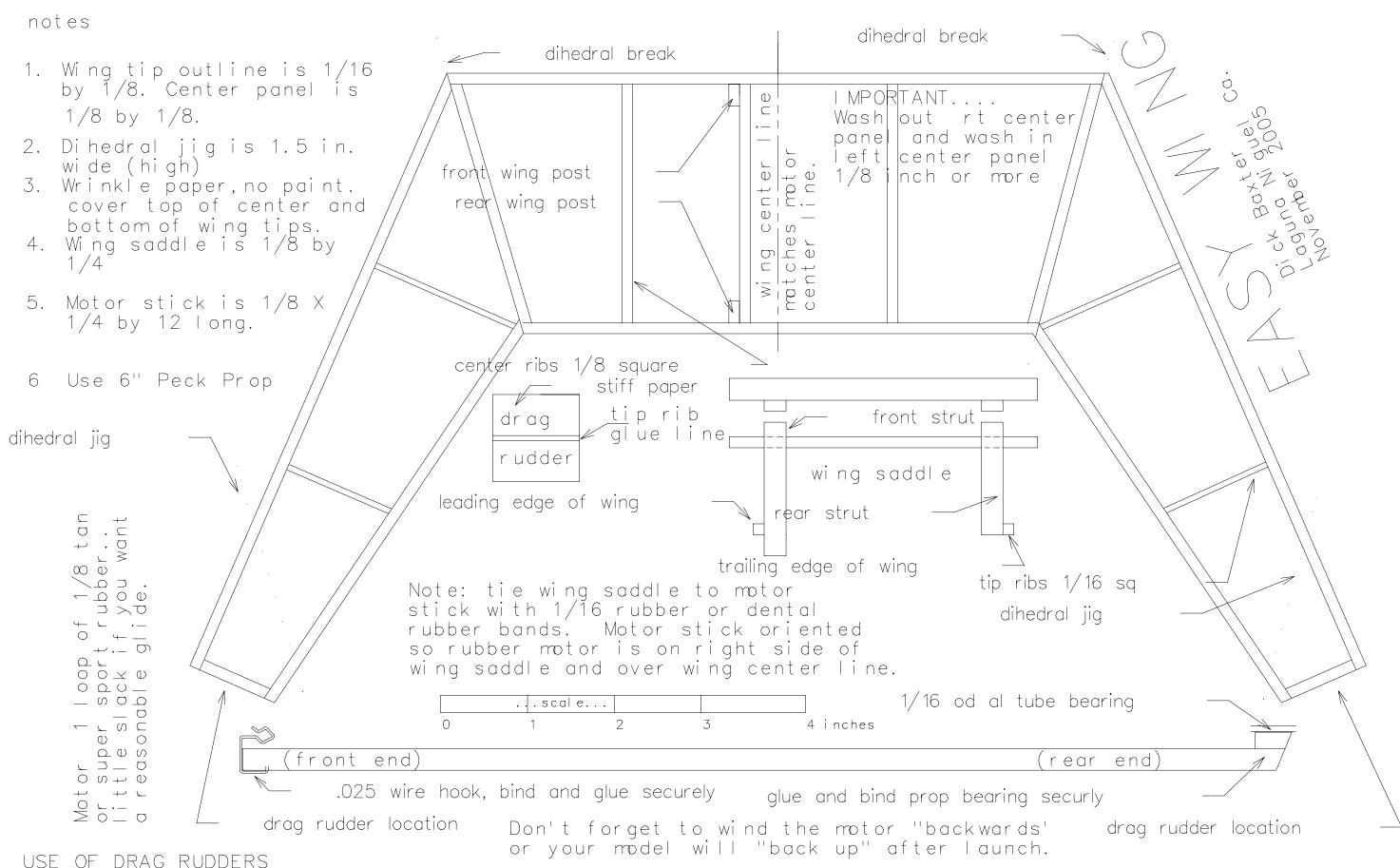
start with both rudders fully retracted (folded flat)...deploy drag rudder on the tip on the INSIDE of the desired turn, by folding the paper perpendicular to the wing surface.
